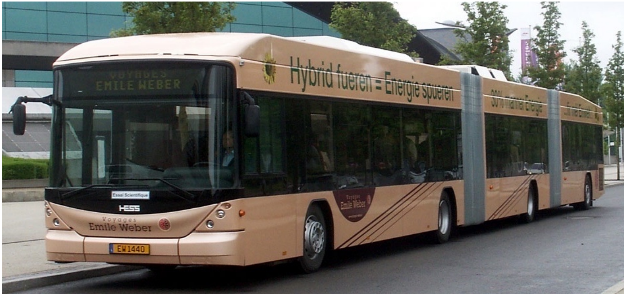
Fig.5 HESS bi-articulated bus
